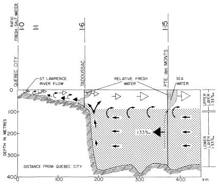
Fig. 7 - Schematic presentation of haline circulation.
